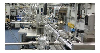
It allows carrying out sample preparation, and reactivity studies under UHV and ambient pressure. Special emphasis is given to the combination of spectroscopy techniques (XPS, UPS, BIS, TPD, HREELS, Kelvin probe) probing the average surface. The system has a modular setup, where the various techniques are mounted in individual chambers, which can be connected to the station on demand. Separation into independent devices ensures robust operation of such complex facility.
